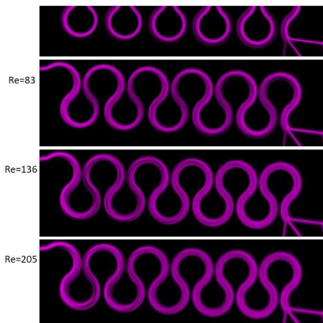
**Figure 4.** Fluids flow in the microchannel with 280° curvature angle at different Reynolds numbers.
