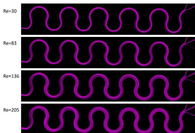
**Figure 3.** Fluids flow in the microchannel with 230° curvature angle at different Reynolds numbers.
