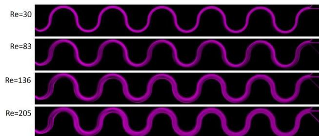
**Figure 2.** Fluids flow in the microchannel with 180° curvature angle at different Reynolds numbers.
