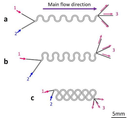
**Figure 1.** Curvilinear microchannels with curvature angles of (a) 180°, (b) 230°, and (c) 280°. 1: Rhodamine B inlet, 2: water inlet, 3: outlet of the mixed fluid.
