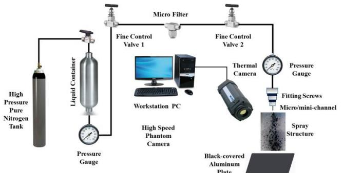
**Figure 1.** Schematic of the Proposed System for Generating Cavitation Bubbles and Micro Cavitating Flows
