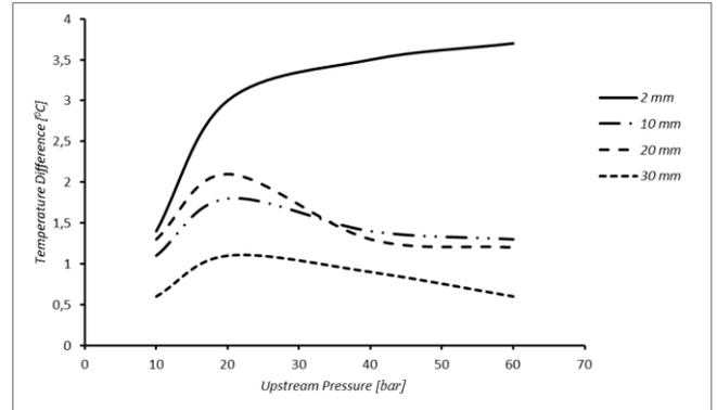
**Figure 4.** Surface temperature rise as a function of upstream pressure for different distance cases at the time of cavitating flow exposure to the target
