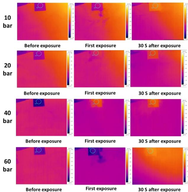
**Figure 3.** The temperature distribution on the targeted plate at the distance of 30 mm from the tip of the nozzle
