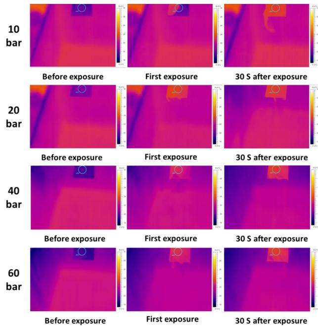
**Figure 2.** The temperature distribution on the targeted plate at the distance of 2 mm from the tip of the nozzle (acquired by the FLIR Thermal camera)
