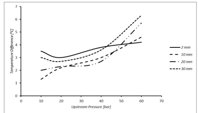
**Figure 5.** Surface temperature rise as a function of upstream pressure for different distance cases 30 seconds after cavitating flow exposure to the target
